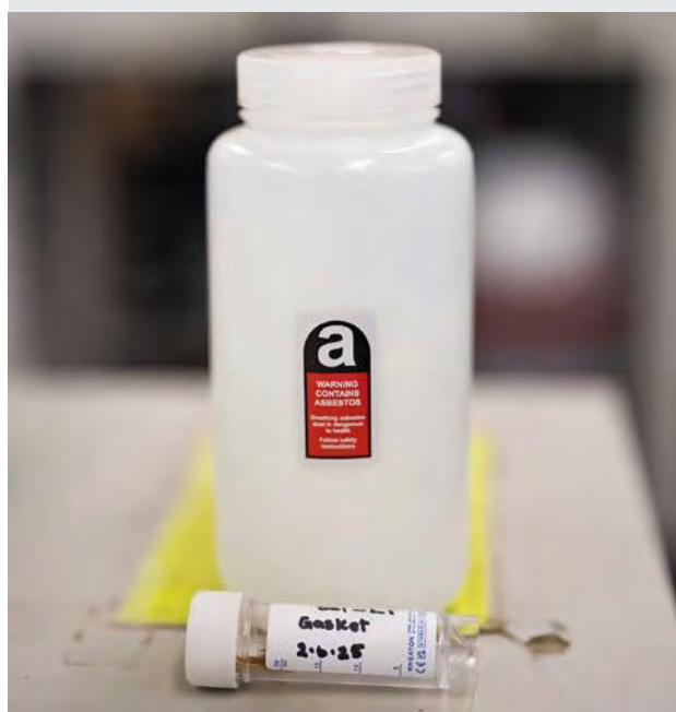
Figure 5-6: Labelling of samples taken for analysis, showing the two-container system
