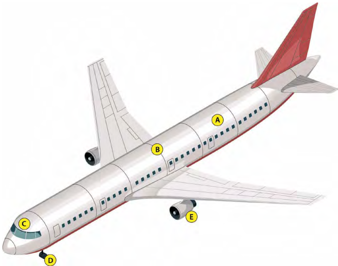
Figure 14-5: Aircraft – where asbestos might be found (non-exhaustive)
